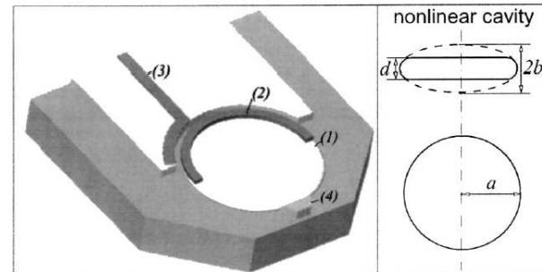
Fig. 1. Experimental setup: (1) LiNbO<sub>3</sub> optical cavity, (2) microwave resonator, (3) microwave feeding stripline, and (4) diaphragm. (Inset) Cross section of the cavity.
