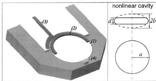
Fig. 1. Experimental setup: (1)  $\text{LiNbO}_3$  optical cavity, (2) microwave resonator, (3) microwave feeding strip line, and (4) diamond coupling prism. Inset: geometric characteristics of the nonlinear optical cavity.
