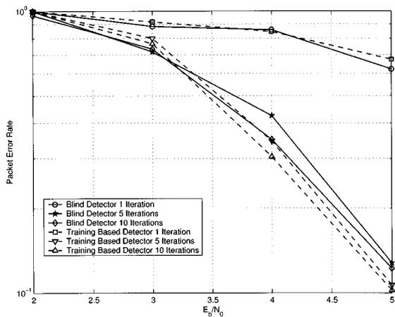
Fig. 4. PER performance comparison for blind detector and training based detector.
