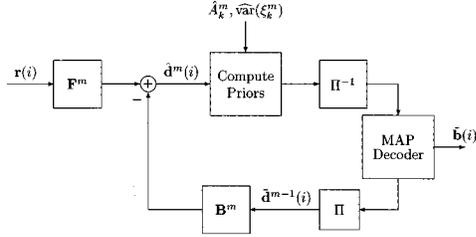
Fig. 2. Structure of the adaptive MMSE iterative P-DFD. The proposed algorithm differs from previous work in the first iteration, when the estimates of  $A_k^m$  and  $\widehat{\text{var}}(\xi_k^m)$  are obtained blindly through the adaptive MOE multiuser detector instead of using training symbols.  $\hat{\mathbf{b}}(i)$  denotes the hard decisions on the information bits.
