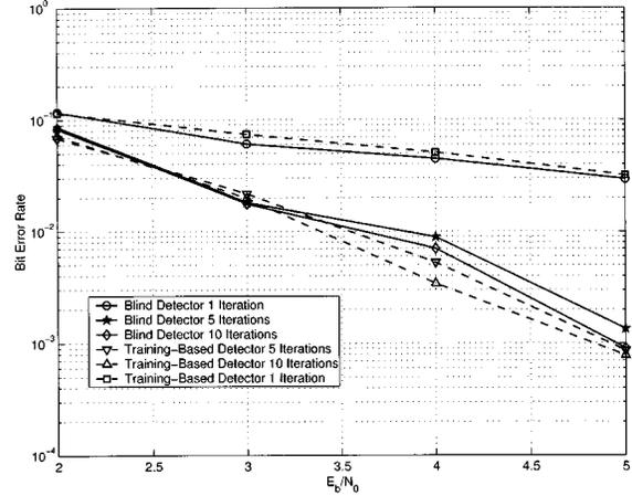
Fig. 3. BER performance comparison for blind detector and training based detector.
