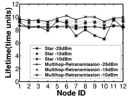
Fig. 12. Network lifetime for different network architectures at different power levels. All environments
