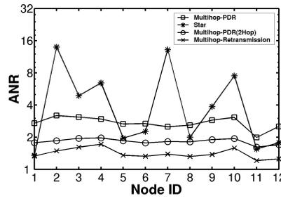
Fig. 8. Average number of retransmissions (ANR) (log base 2 scale) for different architectures. Roof environment. Tx power:  $-25$  dBm
