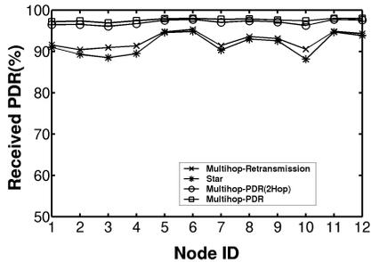
Fig. 4. Received PDR with different network architectures. Lab environment. Tx power:  $-25$   $dBm$ .
