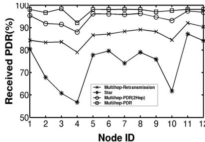
Fig. 5. Received PDR with different network architectures. Roof environment. Tx power:  $-25$   $dBm$ .
