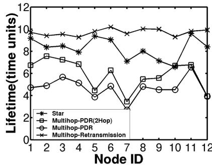
Fig. 11. Network lifetime for different network architectures. All environments. Tx power:  $-25$  dBm
