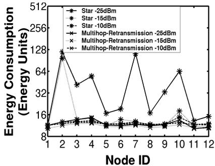
Fig. 10. Energy consumption for star and multihop-retransmissions architectures at different power levels.
