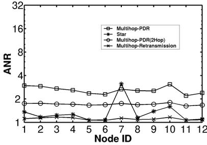
Fig. 7. Average number of retransmissions (ANR) (log base 2 scale) for different architectures. Lab environment. Tx power:  $-25$  dBm
