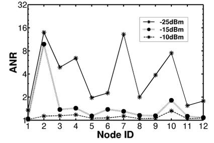
Fig. 9. Average number of retransmissions (ANR) (log base 2 scale) for star architecture at different power levels. Roof environment.
