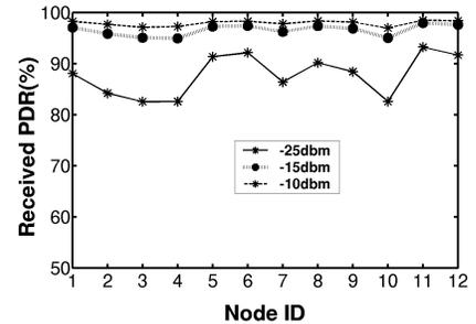
Fig. 6. Received PDR with star architecture at different power levels. All environments.
