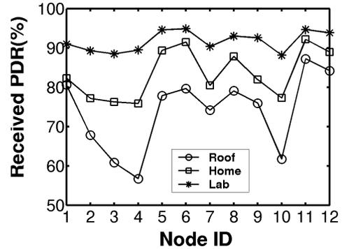
Fig. 2. Received PDR in different environments. Tx power:  $-25\text{ dBm}$ .
