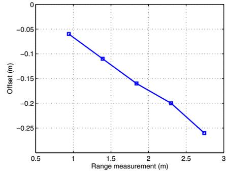
Fig. 9. Error in range measurement vs. reported range.
