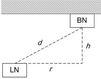
Fig. 4. Original and projected range measurements.
