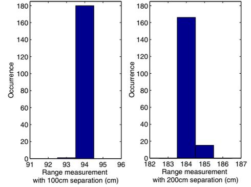
Fig. 8. Histograms for range measurement with 1m (left) and 2m (right) separations.
