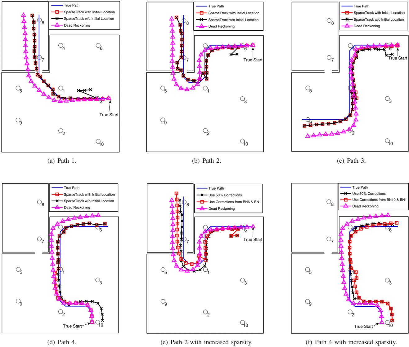
Fig. 11. Figures (a)-(d) present the estimated trajectories for DR and SparseTrack with and without initial location. Figures (e)-(f) present the estimated trajectories with increased sparsity.
