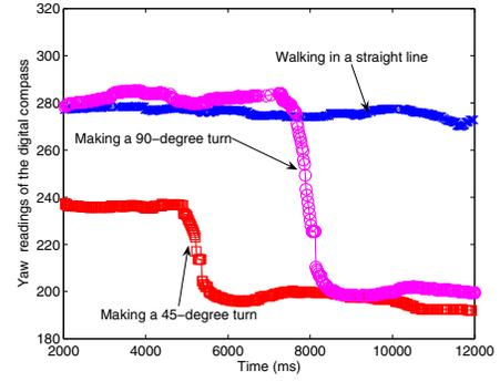
Fig. 7. Yaw readings of digital compass for different walking scenarios.
