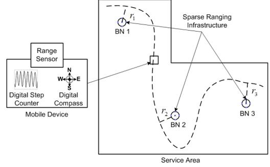
Fig. 5. System architecture of SparseTrack.
