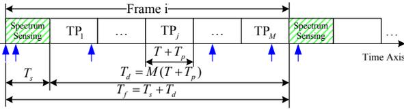
Fig. 2. The designed MAC frame structure for OSA.
