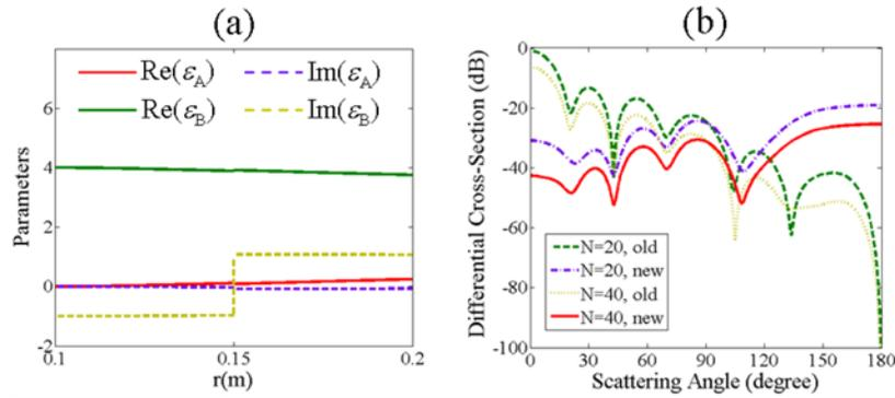
Fig. 4. (a) Constitutive parameters of media-A and media-B along radial direction for isotropic cloak with  $C = 0.5$ . (b) Differential cross section for isotropic cloaks designed by the old set and new set parameter profiles with different layer number ( $N = 20$  and  $N = 40$ ).
