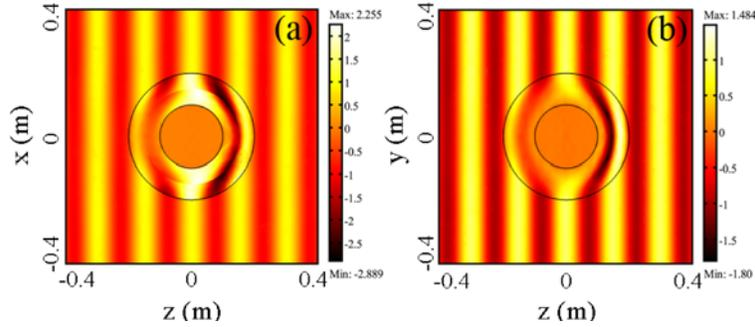
Fig. 2. Snapshots of the total electric field for the spherical gain-assisted cloak with  $C = 0.5$ . (a) x-z plane, (b) y-z plane.
