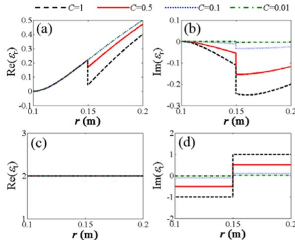
Fig. 1. Permittivity along the radial direction with different  $C$ . (a) Real part of radial parameter. (b) Imaginary part of radial parameter. (c) Real part of transverse parameter. (d) Imaginary part of transverse parameter. The permeability curve will be exactly the same since  $\mu_r = \xi_r$  and  $\mu_t = \xi_t$ , resulting in impedance match.
