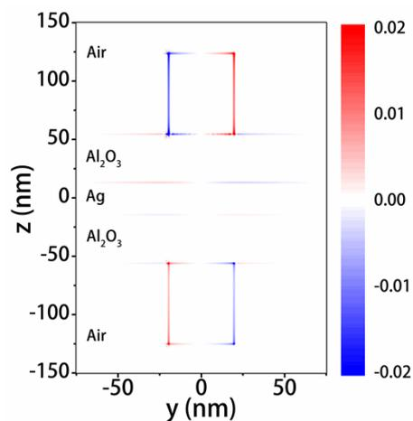
Fig. S1 Charge distribution of one-dimensional nanowire at wavelength  $\lambda = 700$  nm, which supports transmittance as red dashed line shown in Fig. 2d in the main text. It is obvious that dipoles exist on the top and at the bottom. Here  $h = 20$  nm,  $d = 30$  nm,  $t = 50$  nm and  $p_y = 150$  nm.  $L_1 = L_2 = 40$  nm.
