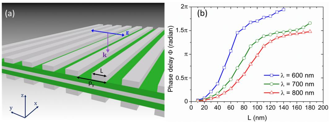
Fig. S2 (a) Schematic structure of one-dimensional nanowire for phase delay estimation and (b) phase delay  $\Phi$  of refracted light versus width of one-dimensional nanowire at wavelength  $\lambda = 600$  nm, 700
