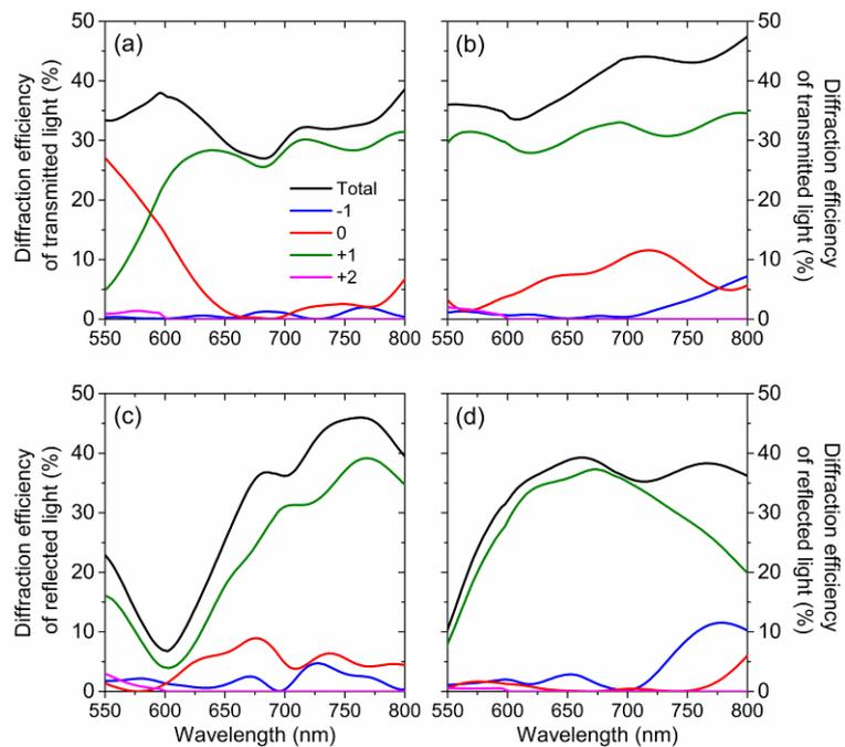
Fig. S4 Diffraction efficiency of transmitted (a) and (b) and reflected (c) and (d) energies against wavelength. (a) and (c) are calculated with  $p_y = 200$  nm while (b) and (d) are calculated with  $p_y = 150$  nm.
