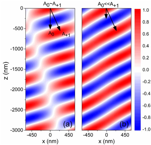
Fig. S5 Interference of 0 and +1 order (anomalous light) for two cases similar to (a)  $p_y = 200$  nm.  $A_0 = 0.37$  and  $A_{+1} = 0.48$  and (b)  $p_y = 150$  nm,  $A_0 = 0.06$  and  $A_{+1} = 0.54$ .
