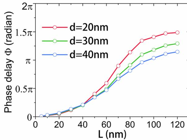
Fig. S6 Phase delay  $\Phi$  of refracted light versus width of one-dimensional nanowire at wavelength  $\lambda = 700$  nm. Here  $h = 20$  nm,  $t = 50$  nm and  $p_y = 150$  nm.  $L_1 = L_2 = L$  ranges from 5 nm to 120 nm.
