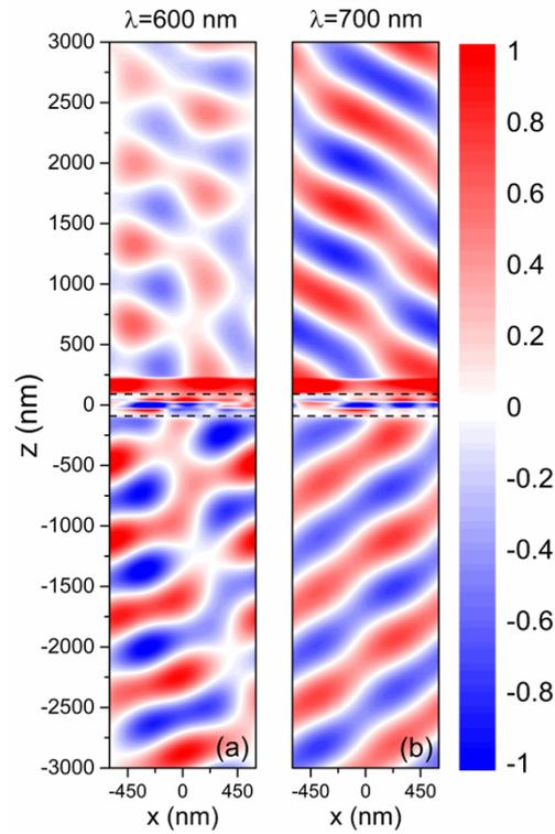
Fig. S3 Electric field distributions of  $E_y$  component at wavelength (a) 600 nm and (b) 700 nm of structure supporting phase delay coverage  $2\pi$  with  $p_y = 200$  nm,  $L_1 = 10$  nm and  $L_2 = 140$  nm. All the simulations are performed at normal incidence. Other parameters are  $h = 20$  nm,  $d = 30$  nm,  $t = 50$  nm and  $p_x = 1200$  nm.
