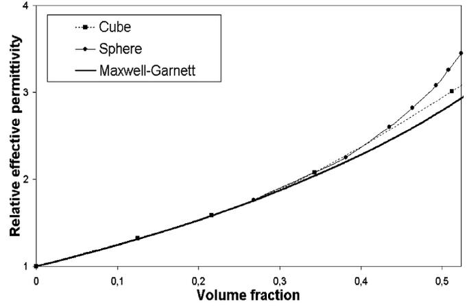
Fig. 7. Effective relative permittivity  $\epsilon_{r\text{eff}}$  for square lattices of spherical and cubical inclusions ( $\epsilon_r = 10$ ) suspended in free space.
