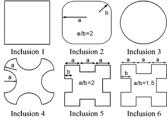
Fig. 2. Geometry of the studied two-dimensional inclusions.
