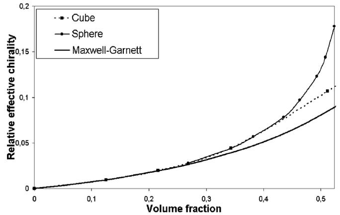
Fig. 8. Effective relative chirality  $\kappa_{\text{eff}}$  for square lattices of spherical and cubical inclusions ( $\kappa = 1$ ) suspended in free space.
