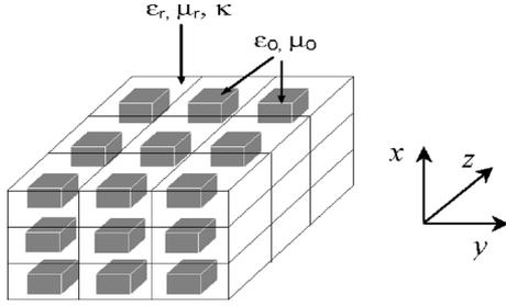
Fig. 9. Finite periodic lattice containing 27 cubical inclusions.
