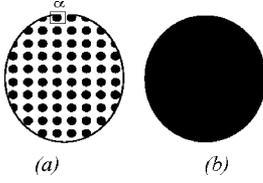
Fig. 1. (a) Periodic composite material. (b) Same material when the periodicity  $\alpha$  tends to zero.
