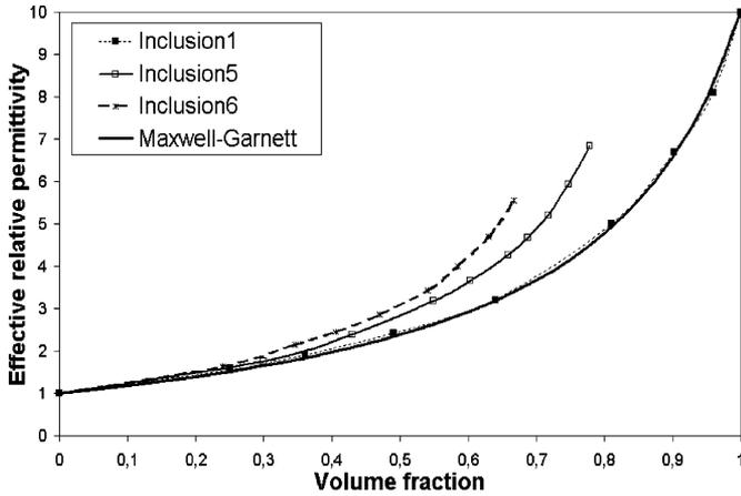
Fig. 5. Effective relative permittivity  $\epsilon_{r\text{eff}}$  for square lattices of inclusions 1, 5, and 6 ( $\epsilon_r = 10$ ) suspended in free space.
