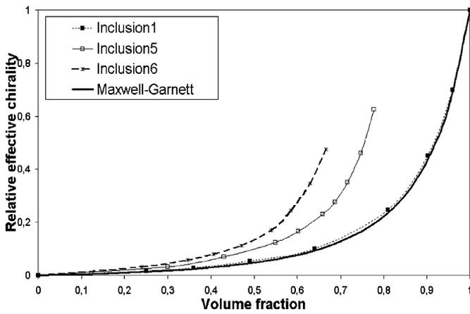
Fig. 6. Computed effective relative chirality  $\kappa_{\text{eff}}$  for square lattices of inclusions 1, 5, and 6 ( $\kappa = 1$ ) suspended in free space.
