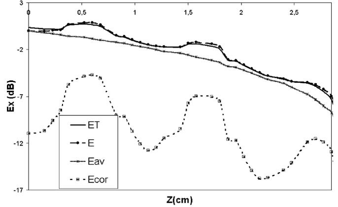
Fig. 10. Magnitude of the  $x$ -component of the electric field as a function of position along  $z$ -axis at  $x = y = L/2$
