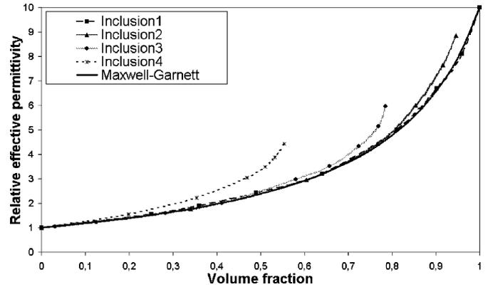
Fig. 3. Computed effective relative permittivity  $\varepsilon_{\text{reff}}$  for square lattices of inclusions 1–4 ( $\varepsilon_r = 10$ ) suspended in free space.
