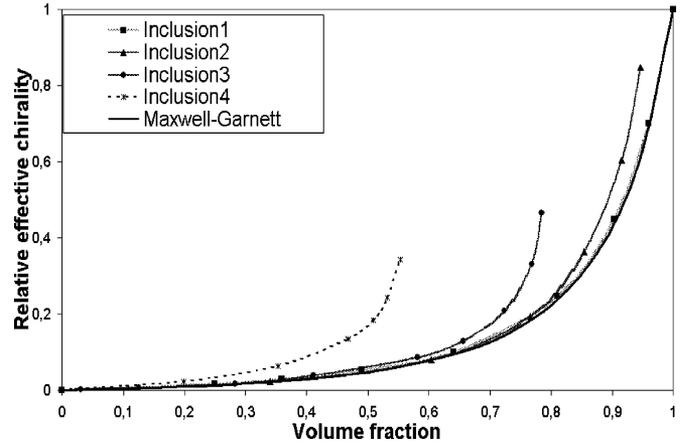
Fig. 4. Effective relative chirality  $\kappa_{\text{eff}}$  for square lattices of inclusions 1–4 ( $\kappa = 1$ ) suspended in free space.
