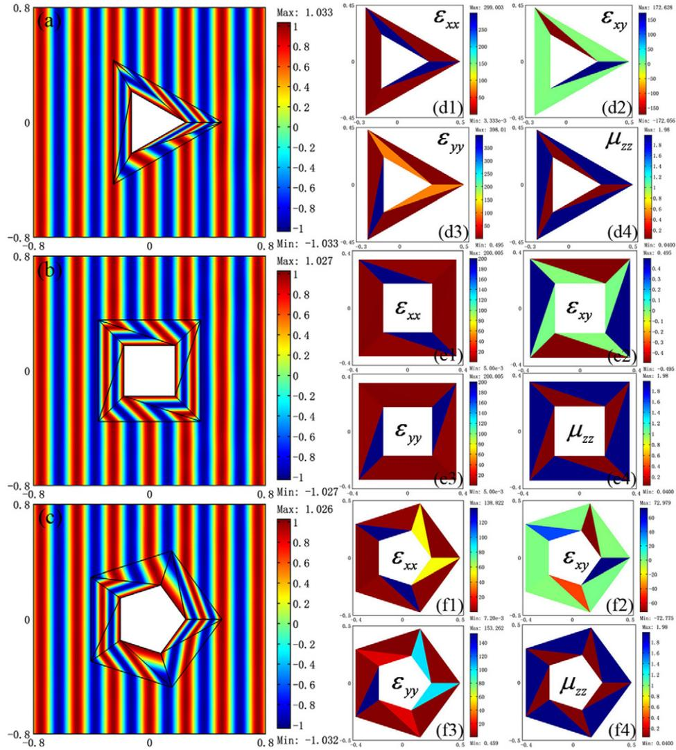
**Figure 2.** The snapshots of the total magnetic fields ((a)–(c)) and parameter distributions ((d)–(f)) for the symmetrical polygonal cloaks. ((a), (d)) The three-sided polygonal cloak. ((b), (e)) The four-sided polygonal cloak. ((c), (f)) The five-sided polygonal cloak.
