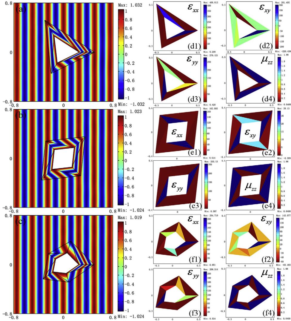
**Figure 3.** The snapshots of the total magnetic fields ((a)–(c)) and parameter distributions ((d)–(f)) for the asymmetrical polygonal cloaks. ((a), (d)) The three-sided polygonal cloak. ((b), (e)) The four-sided polygonal cloak. ((c), (f)) The five-sided polygonal cloak.
