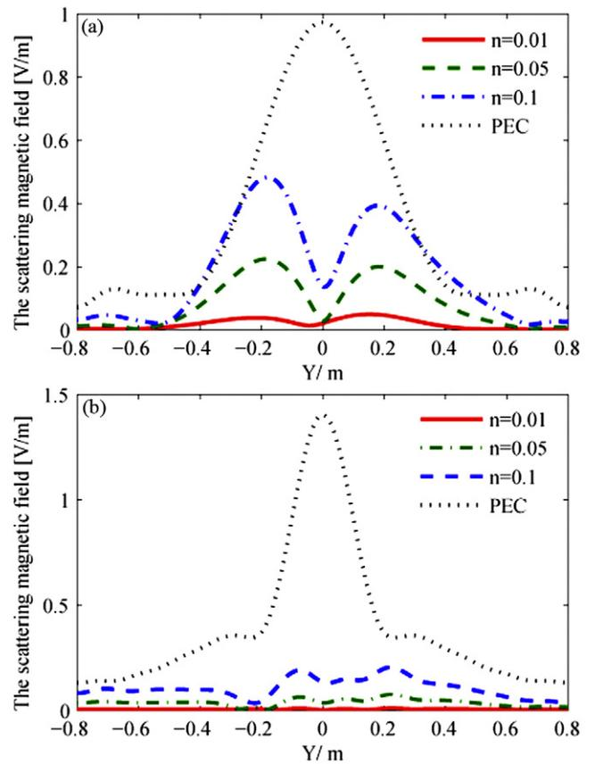
**Figure 4.** The comparison of the scattered magnetic fields for a three-sided symmetrical polygonal PEC case with or without the cloak for different values of  $n$ . (a) The forward scattering at the observation line  $x = 0.6$  m. (b) The backward scattering at the observation line  $x = -0.4$  m.
