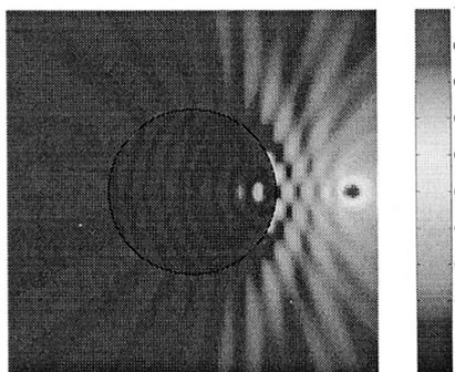
**Fig. 7** Normalized magnitude of Poynting vector of a bi-isotropic cylinder of  $a = 2.5\lambda$  filled with chiral nihility medium of  $\epsilon_r = 1e-5$ ,  $\mu_r = 1e-5$ , and  $\kappa = 1$  and the line source at  $(4.8\lambda, 0^\circ)$ .
