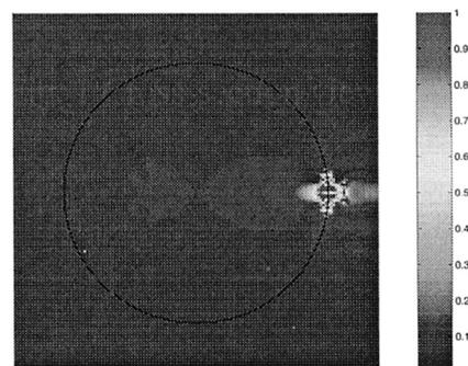
**Fig. 2** Normalized magnitude of Poynting vector of a cylinder of  $a = 4\lambda$  filled with anti-vacuum and the line source at  $(4.5\lambda, 0^\circ)$ .
