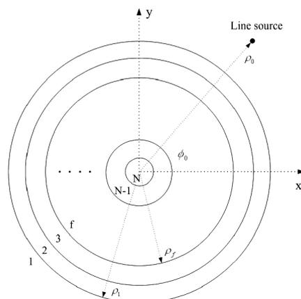
**Fig. 1** Cross-section view of a multilayered cylinder with the line source in 1st region.
