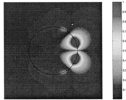
**Fig. 5** Normalized magnitude of Poynting vector of a cylinder of  $a = 0.05\lambda$  filled with anti-vacuum and the line source at  $(0.25\lambda, 0^\circ)$ .
