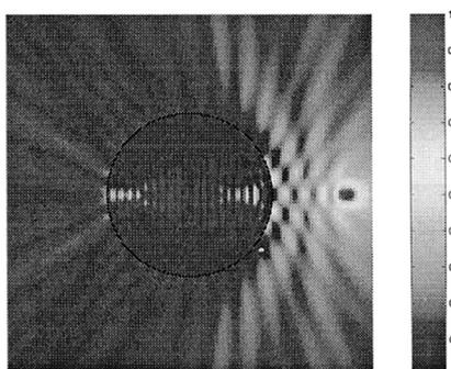
**Fig. 8** Normalized magnitude of Poynting vector of a cylinder of  $a = 2.5\lambda$  filled with bi-isotropic medium of  $\epsilon_r = 1$ ,  $\mu_r = 1$ , and  $\kappa = 2$  and the line source at  $(4.8\lambda, 0^\circ)$ .
