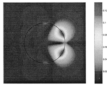
**Fig. 6** Normalized magnitude of Poynting vector of a cylinder of  $a = 0.05\lambda$  filled with anti-vacuum and the line source at  $(1.05\lambda, 0^\circ)$ .
