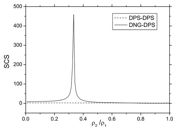
**Fig. 11** Scattering cross section versus ratio of core layer over cloaking layer in two pairs of combinations: DNG-DPS and DPS-DPS. In the case of DNG-DPS pairing, the cloaking layer is filled with DNG medium of  $(-3\epsilon_0, -2\mu_0)$ , and in the case of DPS-DPS pairing, the cloaking layer is filled with DPS medium of  $(3\epsilon_0, 2\mu_0)$ . The core layer remains the same DPS medium of  $(2\epsilon_0, \mu_0)$  for both pairings.
