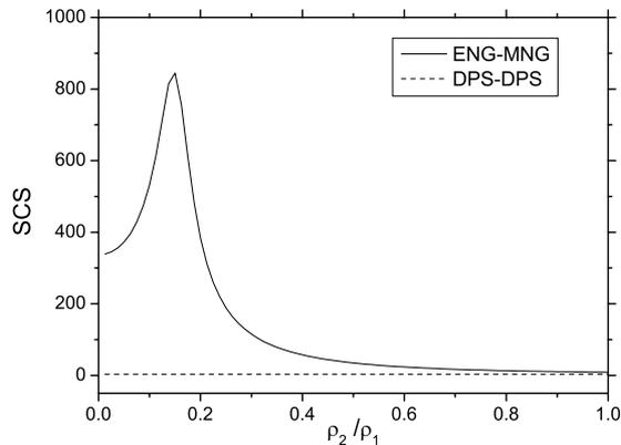
**Fig. 12** Scattering cross section versus ratio of core layer over cloaking layer in two pairs of combinations: ENG-MNG and DPS-DPS. In the case of ENG-MNG pairing, the cloaking layer is filled with ENG medium of  $(-3\epsilon_0, \mu_0)$ , while core layer is occupied by MNG medium of  $(4\epsilon_0, -2\mu_0)$ . In the case of DPS-DPS pairing, the cloaking and core layers are filled with DPS medium of  $(3\epsilon_0, \mu_0)$  and  $(4\epsilon_0, 2\mu_0)$ , respectively.
