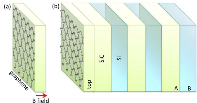
FIG. 1. (a) A schematic diagram of a double-layer structure consisting of graphene and SiC substrate and (b) one-dimensional graphene-based PC structure. An external magnetic field is indicated by an arrow, which is perpendicular to graphene.
