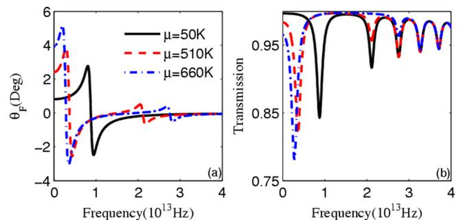
FIG. 2. Dependence of FR angle of the double-layer structure on frequency and chemical potential. (a) FR angle as a function of frequency at  $\mu = 50$  K (solid line), 510 K (dash line), and 660 K (dash-dotted line), respectively. (b) Transmission as a function of frequency with the same chemical potentials in Fig. 2(a).
