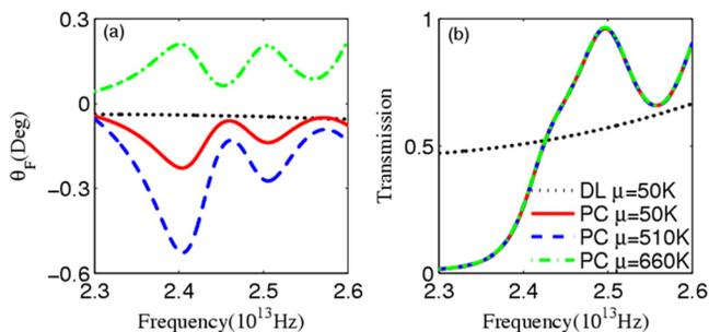
FIG. 3. Dependence of FR angle of the hybrid structure on frequency and chemical potential. (a) FR angle (b) transmission as a function of frequency with the same chemical potentials used in Fig. 2. The results of the double-layer structure (dotted line) are also shown for comparison.
