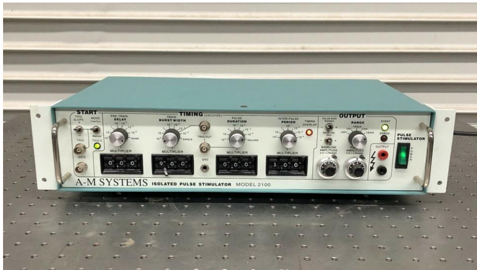
Figure S 3. A photo of a commercial stimulator (AM System 2100 isolated pulse stimulator)
