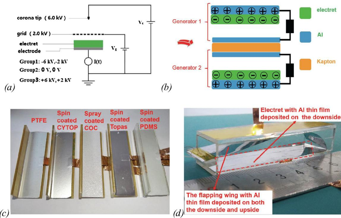
**Fig. 2.** (a)The corona charging setup for electret materials; (b) The structure of E-TriG with two Al-electret pairs for generator 1 (top) and generator 2 (bottom); (c) Image of the electret films and their application in E-TriG: from left to right: PTFE film, spin coated CYTOP film, spray coated COC film, spin coated Topas film and PDMS film; (d) An E-TriG device is assembled with a flapping wing and two counter electret films. The overall size of the E-TriG is 67 mm × 22 mm × 10 mm.
