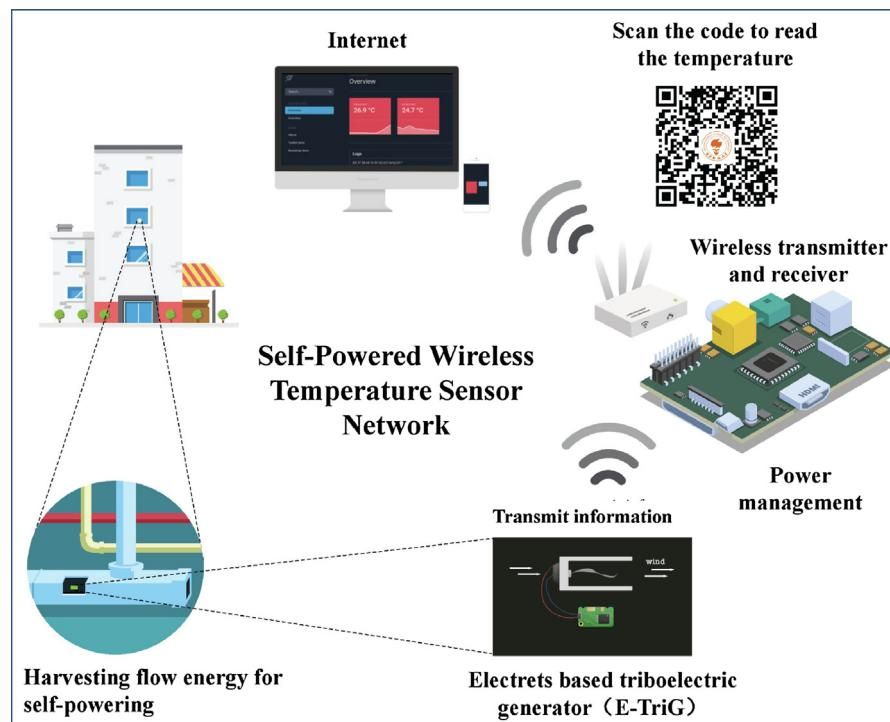
**Fig. 1.** Schematic map of the self-powered wireless temperature sensing system to monitor the temperature of the central air conditioning system, with the energy scavenging from the air flow.
