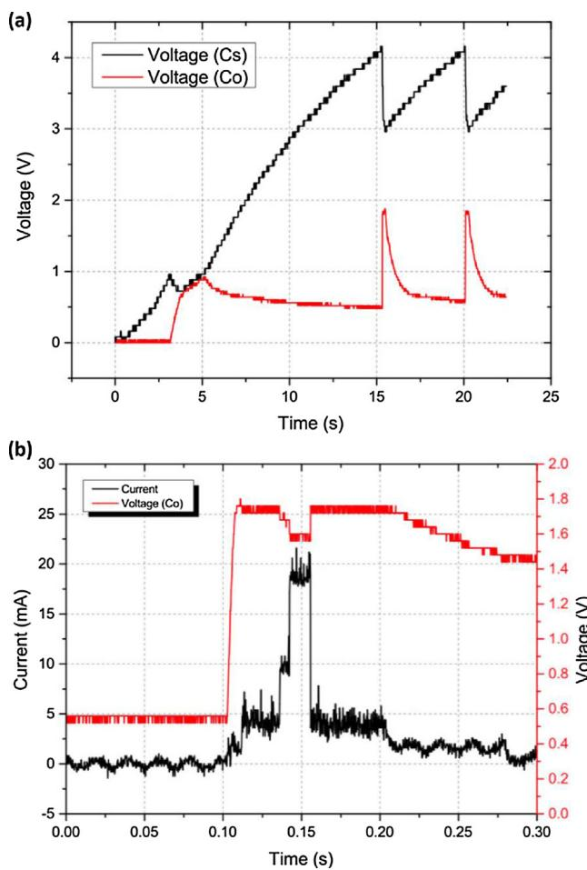
**Fig. 8.** (a) V-t curves for Cs for energy storage and Co for providing a trigger signal to set the mode of the power management; (b) Closed-up view of the voltage and current of Co, showing the generation of the trigger signal.
