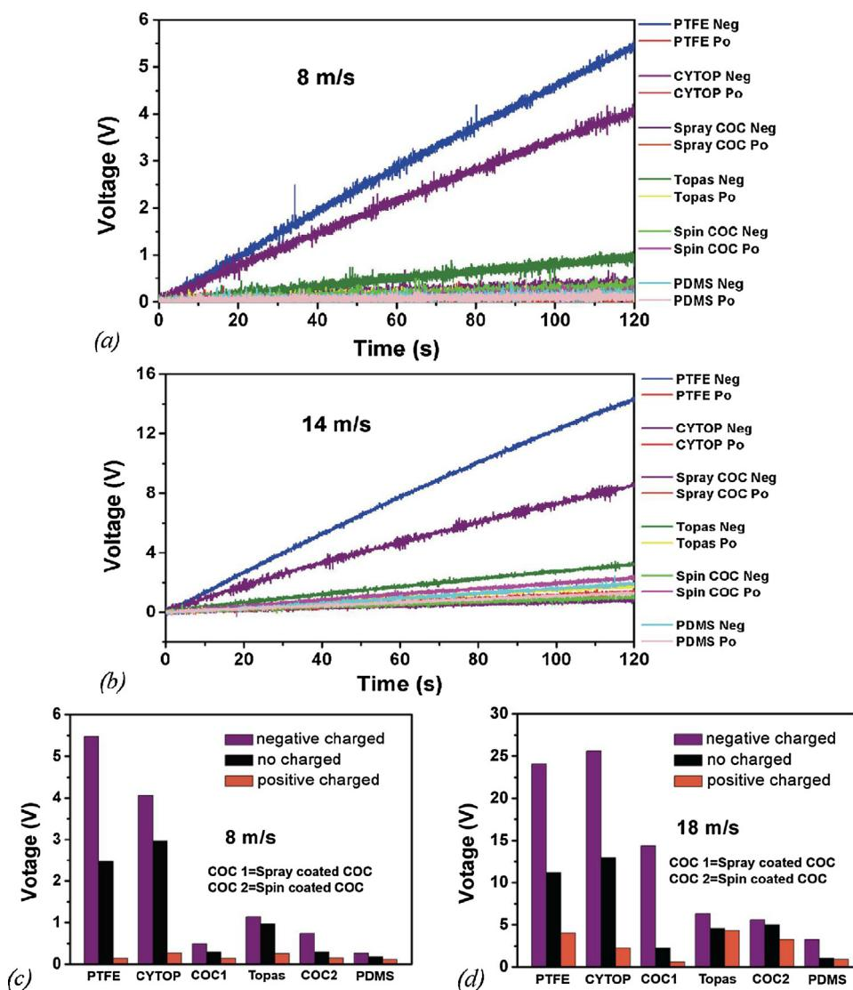
**Fig. 6.** Capacitor charging performance from E-TriG devices under different wind speeds of (a) 8 m/s; (b) 14 m/s with electret materials of PTFE; CYTOP; Spray-coated COC (COC1); Spin-coated TOPAS; Spin-coated COC (COC2) and PDMS; (c,d) Statistic comparison among the electrets with different charging conditions with wind speeds of 8 m/s and 18 m/s, respectively.
