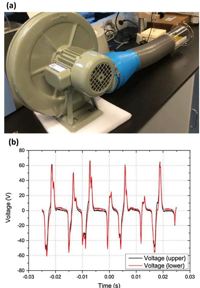
**Fig. 4.** (a) An air blower is used to generate the wind flow, and a commercial anemometer is used to monitor the flow rate during the measurement. (b) Open circuit voltage output of one E-TriG prior to rectifying. Each E-TriG device is composed of an upper device (generator 1) and a lower device (generator 2), which can improve the overall power output. It should be noted that the voltage signal of the lower device is mirrored top-down for better comparison.
