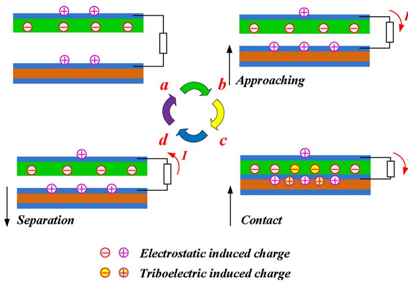
**Fig. 3.** The function mechanism of the electret enhanced triboelectric generator.
