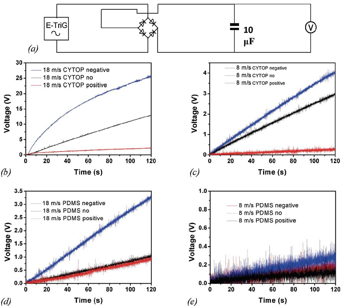
**Fig. 5.** (a) Test circuit for the E-TriG with a rectifier and charging capacitor; Capacitor charging performance from E-TriG devices with electret materials of (b–c) CYTOP; (d,e) PDMS under two wind speeds of 18 m/s and 8 m/s, respectively.
