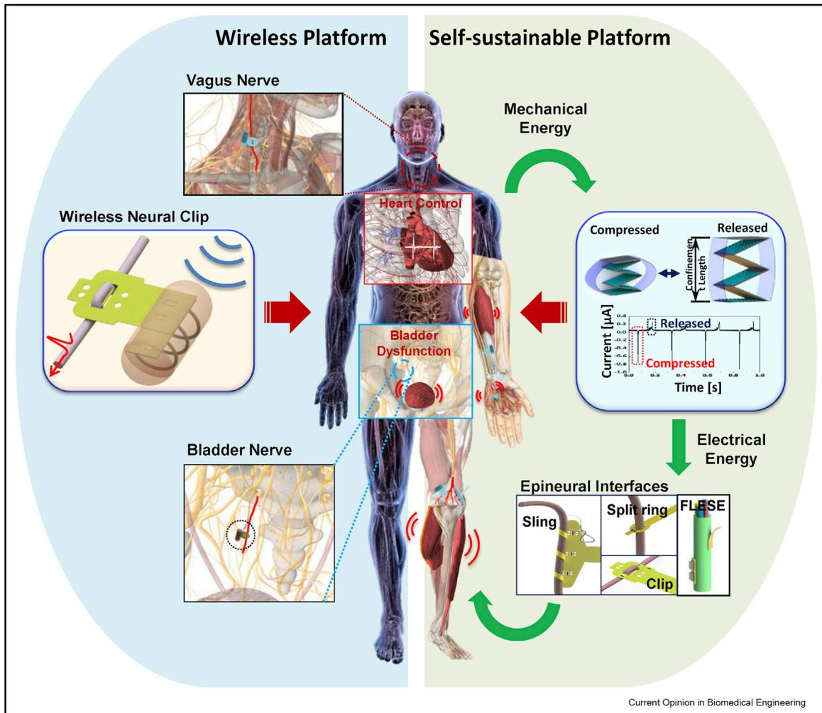
Schematic diagram of wireless and self-sustainable platforms for advanced neural interfaces and their applications.
