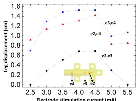
**Fig. 9.** Correlation between electrode stimulation current and leg displacement (mean value of 20 displacements). For a certain subset of electrode, the leg displacement tends to increase with the stimulation current at first, and then saturate, followed by dropping at large stimulation current.
