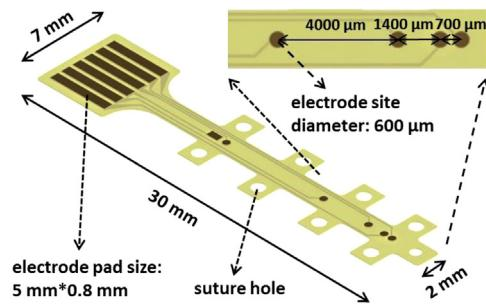
**Fig. 1.** Schematic illustration of device design. Six electrodes of same diameter are distributed with uneven distance between each other. Two arrays of suture holes facilitate the fixation of the device on the target muscle.
