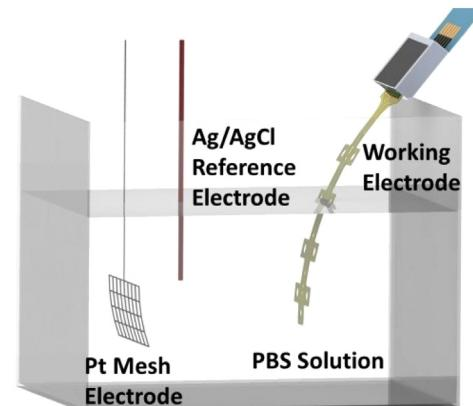
**Fig. 4.** Three-electrode setup. The working electrode, Ag/AgCl reference electrode, and Pt mesh electrode are immersed into the PBS solution.
