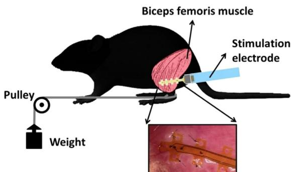
**Fig. 8.** Illustration of in-vivo muscle stimulation. The device is sutured to Biceps femoris muscle surface. A weight is tied to the leg through a pulley system. By recording the vertical movement of the weight, the leg displacement can be derived.
