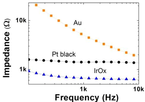
**Fig. 6.** Bode plot of electrode impedance. At 1 KHz, IrOx shows lower impedance of 0.7 kΩ, compared to Pt black of 1.4 kΩ and gold of 5.3 kΩ.
