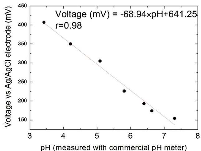
**Fig. 7.** pH calibration of IrOx electrode and commercial glass pH meter. Open circuit voltage shows linear relationship with the pH change.
