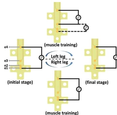
**Fig. 10.** Experiment design for comparison of muscle fatigue using different electrode pairs. During the muscle fatigue induce process, the left leg is stimulated with alternating electrode pairs, while the right leg is stimulated with fixed electrode pair.
