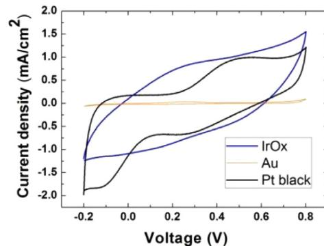
**Fig. 5.** Cyclic Voltammograms (CV) of different contact materials. The current density is derived from dividing the current by interface electrode area.
