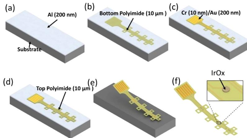
**Fig. 2.** Fabrication process. The device is fabricated layer by layer on the silicon substrate, and then released by etching away the aluminium sacrificial layer.
