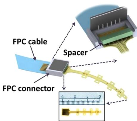
**Fig. 3.** Schematic illustration of the device connected to a FPC connector. The pads on the device are designed to match the FPC connector, and can be plugged in the FPC connector easily.
