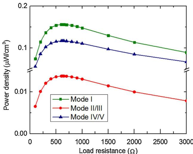
**Fig. 9.** Output power density versus various load resistances for the three vibration frequencies of 840 (mode I), 1070 (mode II/III) and 1490 (mode IV/V) Hz.
