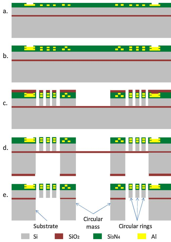
**Fig. 3.** Micro-fabrication processes of the EH chip.
