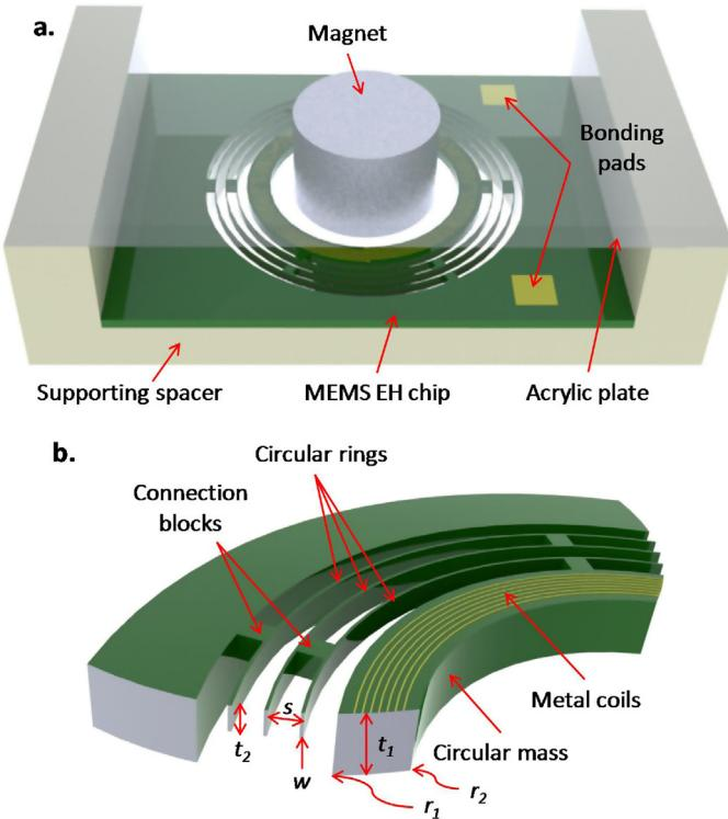
**Fig. 1.** Schematic drawing of the multi-frequency MEMS electromagnetic EH device.
