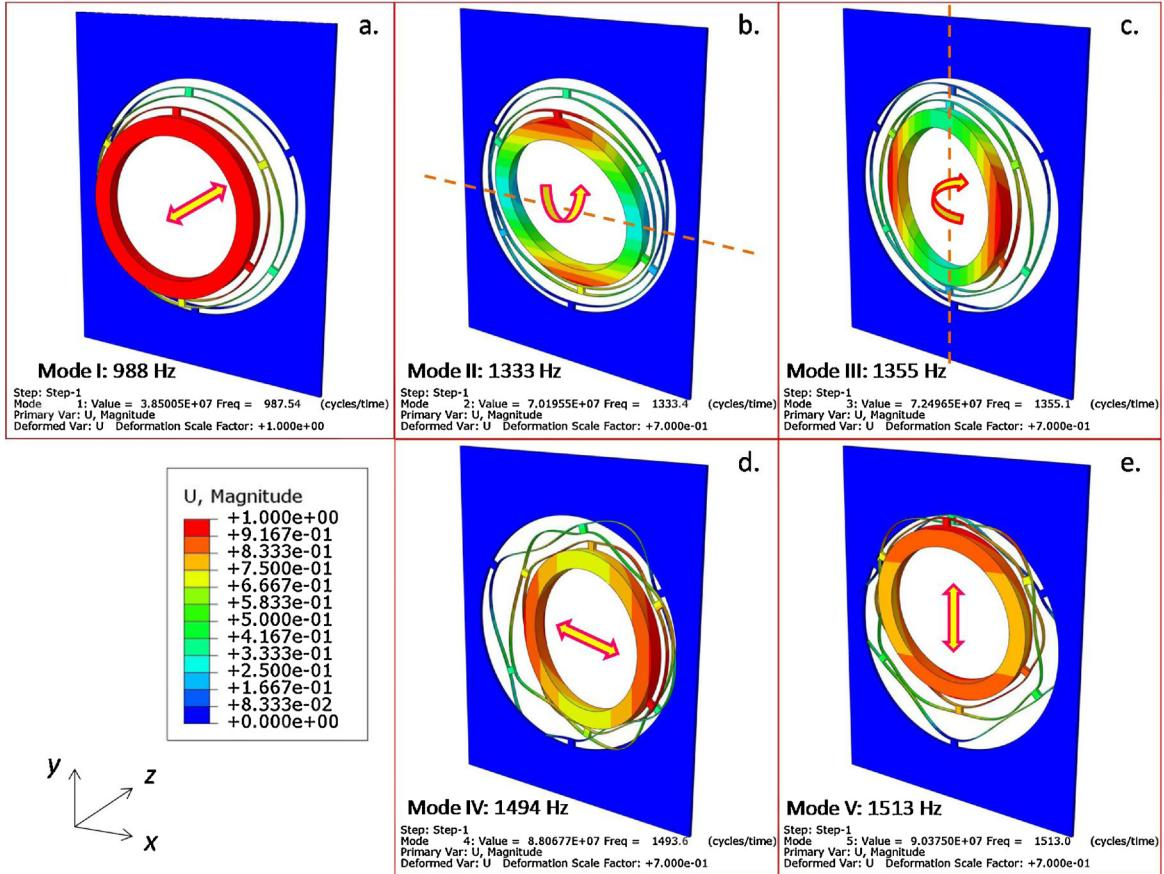
**Fig. 2.** Finite element analysis results: (a) mode I at 988 Hz; (b) mode II at 1333 Hz; (c) mode III at 1355 Hz; (d) mode IV at 1494 Hz and (e) mode V at 1513 Hz.
