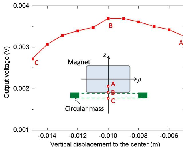
**Fig. 7.** Output voltage of the EH device against the vertical displacement of the circular mass from -0.5 to -1.5 mm at vibration mode I.
