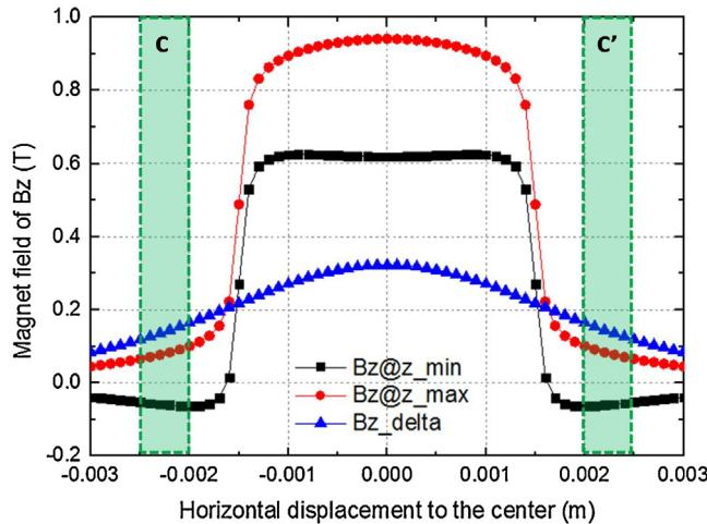
**Fig. 6.** Magnetic field component  $B_z$  and the change of the magnetic field  $B_z_{\delta}$  for the peak-to-peak vibration displacement of the moving coils experienced.
