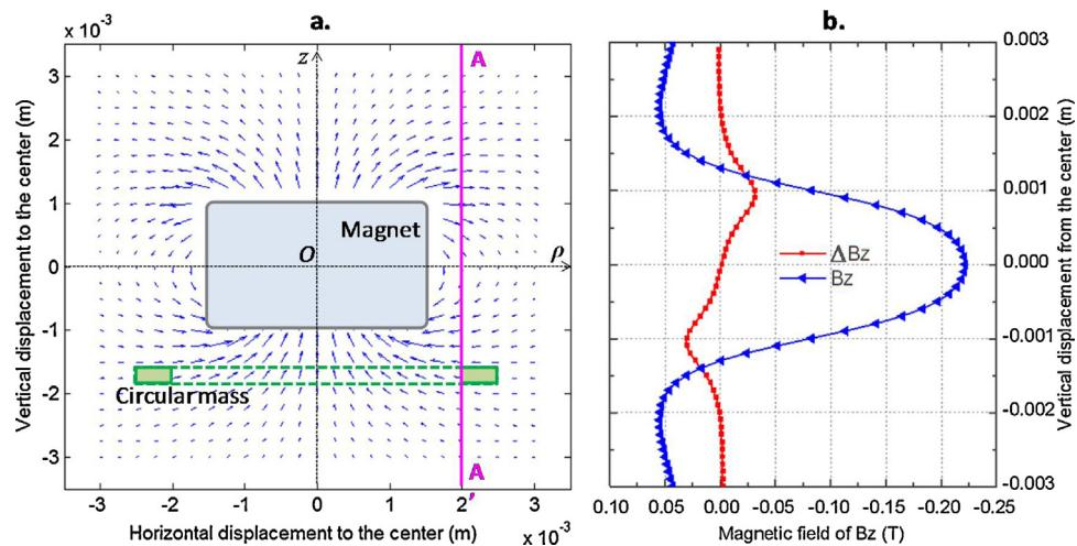
**Fig. 5.** (a) Magnetic field distribution around a cylinder magnet of 2-mm-height and 1.5-mm-radius; (b) magnetic field component  $B_z$  and magnetic field change  $\Delta B_z$  against the vertical displacement for a fixed horizontal displacement of 2 mm.
