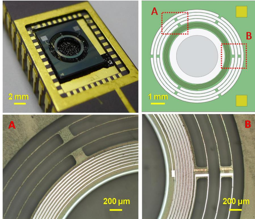
**Fig. 4.** (a) Photograph of the micro-fabricated EH chip assembled onto a DIP; (b) enlarged views of parts A and B of the EH chip taken by microscope.
