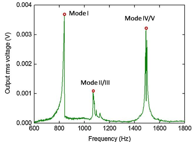
**Fig. 8.** Output voltage of the EH device against the excitation frequency sweeping from 600 to 1800 Hz at 1.0 g.
