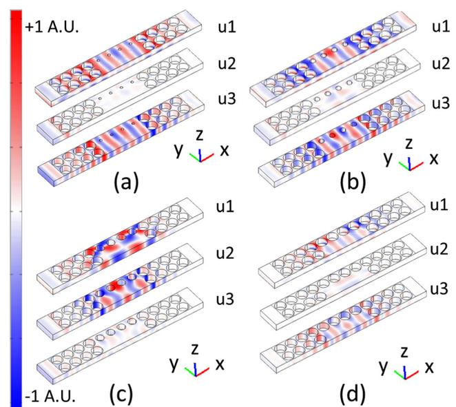
FIG. 3. (Color online) Simulated mode profiles of displacement of PnC resonators with alternate defects and with (a)  $r' = 2 \mu\text{m}$  (b)  $r' = 4 \mu\text{m}$  (c)  $r' = 6 \mu\text{m}$  (d)  $r' = 8 \mu\text{m}$ . The  $u_1$ ,  $u_2$ , and  $u_3$  represent the displacement vector components in  $x$ ,  $y$ , and  $z$  directions, respectively. The color bar indicates the amplitude of displacements in an arbitrary unit.
