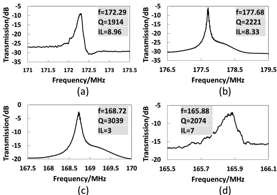
FIG. 2. Measured transmission spectra of PnC resonators with alternate defects and with (a)  $r' = 2 \mu\text{m}$  (b)  $r' = 4 \mu\text{m}$  (c)  $r' = 6 \mu\text{m}$  (d)  $r' = 8 \mu\text{m}$ .  $f$ ,  $Q$ ,  $IL$  refer to the resonant frequency, the  $Q$  factor, and the insertion loss of the PnC resonator, respectively.
