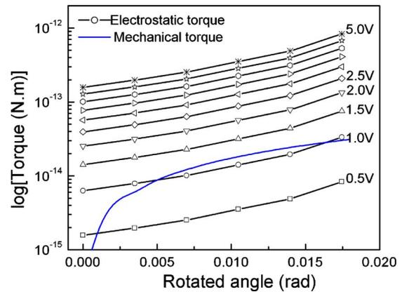
FIG. 4. (Color online) The mechanical torque and the electrostatic torque applied on a model of NEMS torsion switch. In this NEMS switch model, TL is 1.5  $\mu\text{m}$ , TW is 200 nm, CL is 2  $\mu\text{m}$ , and CW is 1.5  $\mu\text{m}$ , the thickness of torsion spring is 70 nm and the distance between the free end of cantilever and bottom electrode is 50 nm.
