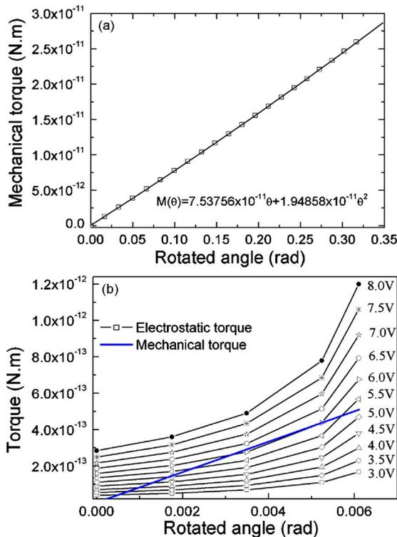
FIG. 3. (Color online) (a) The simulated mechanical torque-rotated angle for the NEMS torsion switch. In the initial state, the torsion bar has not been pretwisted. (b) The mechanical torque and the electrostatic torque applied on the fabricated NEMS torsion switch. In the initial state, the torsion bar is assumed to be pretwisted for 0.207 rad.
