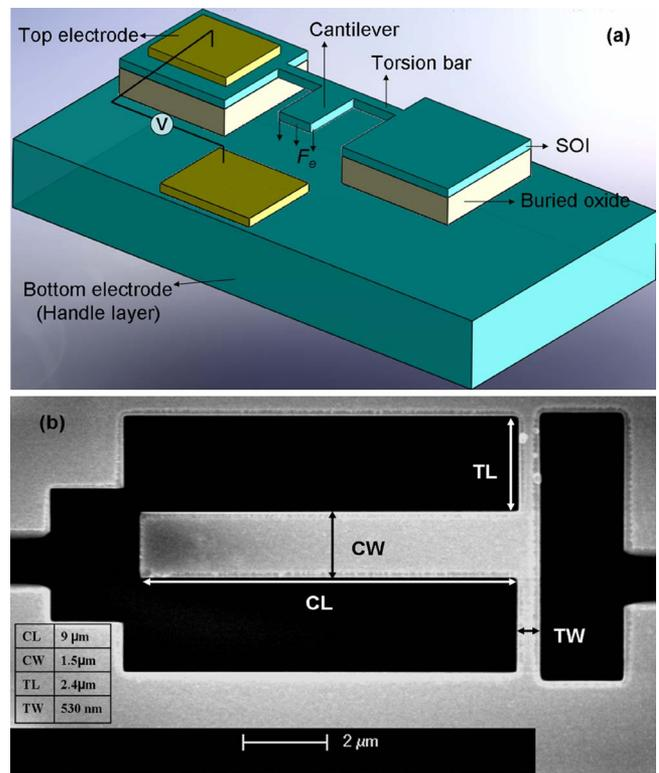
FIG. 1. (Color online) (a) A schematic illustration of the NEMS torsion switch device. (b) SEM photo of a NEMS torsion switch after HF vapor releasing. The CL, CW, TL, and TW of device are 9  $\mu\text{m}$ , 1.5  $\mu\text{m}$ , 2.4  $\mu\text{m}$ , and 530 nm, respectively.
