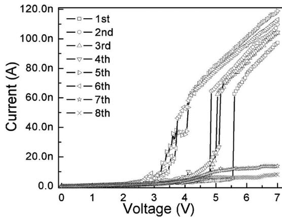
FIG. 2.  $I$ - $V$  characteristic of the device shown in Fig. 1(b) in multiple operations.
