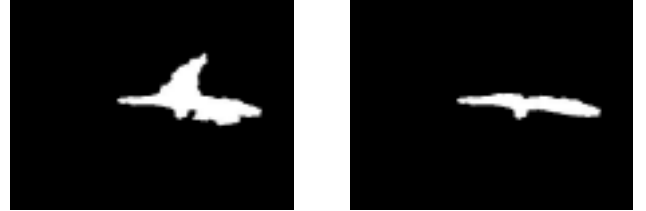
a. Independent object segmentation without MRF b. Independent object segmentation with MRF
