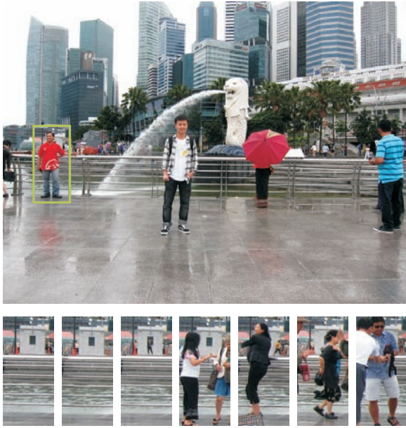
Figure 3: Correlation comparison used to detect unobstructed patches. The ROI is outlined in the green rectangle in the current view, the bottom row of figures are 7 patches warped from reference images, ranked according to average NCC scores.
