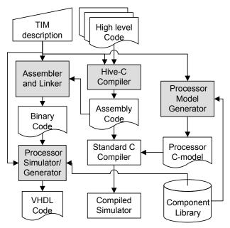
Figure 1. Silicon Hive design flow
