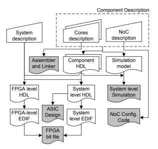
Figure 6. Integrated flow for system development (design-time)
