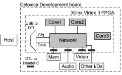
Figure 5. Architecture of the reconfigurable system
