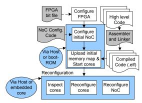
Figure 7. Run-time flow for (re-)configuration
