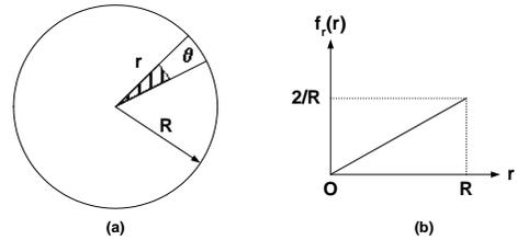
Fig. 1. Probability distribution of one-hop distance  $r$ . In (a) we illustrate how to derive its probability distribution function from the ratio of the sector area. The shape of its probability density function is shown in (b).
