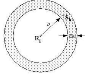
Fig. 2. The concentric ring model. The space is divided into infinite non-overlapping concentric rings centered at  $R_i$ . Each ring can hold at most one active sender. The aggregate interference at  $R_i$  is the summation of the power level received from the active sender inside each ring, if any.
