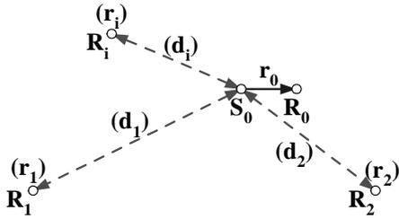
Fig. 3. The node cloud model.  $S_0$ - $R_0$  is a transmission pair placed with other active nodes in a node cloud. The  $r_i$  in parenthesis is the one-hop distance associated with the active receiver  $R_i$ . The  $d_i$  on the edge denotes the distance from  $S_0$  to  $R_i$ .
