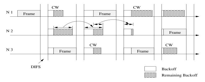
Fig. 3. The backoff mechanism of 802.11 MAC (based on Figure 3 of [29]). The frame transmission time includes the RTS/CTS exchange and the MAC layer ACK. CW = Contention Window.
