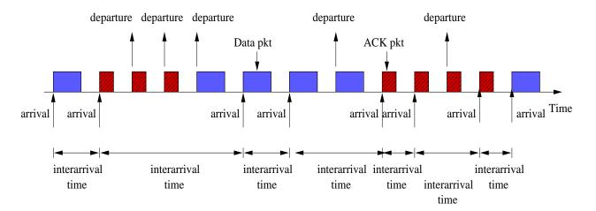
Fig. 5. Packet arrivals and departures at node B with bi-directional data flow.
