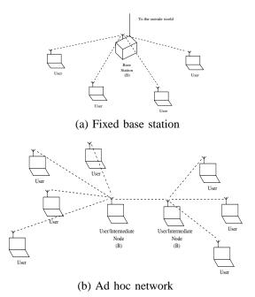
Fig. 2. The network models assumed in this paper: (a) shows a BSS with a fixed base station while (b) considers an ad hoc network.
