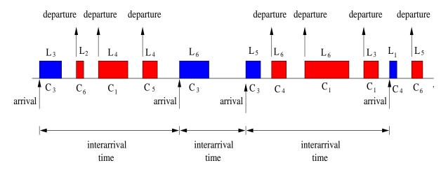
Fig. 6. Packet arrivals and departures at node B with multirate data flow.
