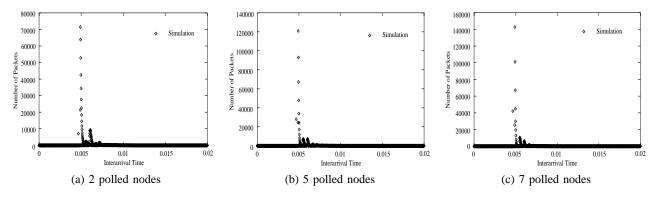
Fig. 13. Interarrival times with PCF operation with 10 nodes. (Superframe size = 500msec, 1000 byte packets)
