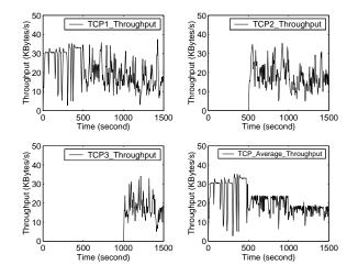
Fig. 6. Throughput and Average Per-Flow Throughput of TCP Sessions
