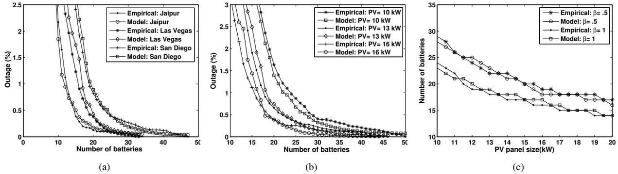
Fig. 5. (a) Outage vs number of batteries required for a PV wattage of 12 kW (b) Outage vs batteries required for various PV panel sizes: San Diego (c) Number of batteries vs PV wattage required for different outage probabilities ( $\beta$ ): San Diego.
