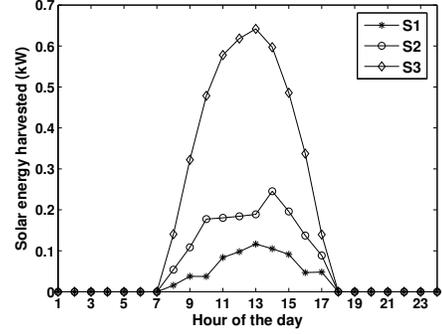
Fig. 1. Average hourly values of the solar energy harvested for the 3 day types for the Month of February for San Diego (PV panel rating = 1 kW)
