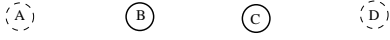
Fig. 5. Senders B and C may transmit at the same time without causing collisions. However, one of them still needs to withdraw to avoid a potential future collision that involves their receivers' acknowledgment packets.
