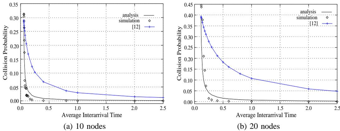
Fig. 2. Comparison of the collision probabilities.
