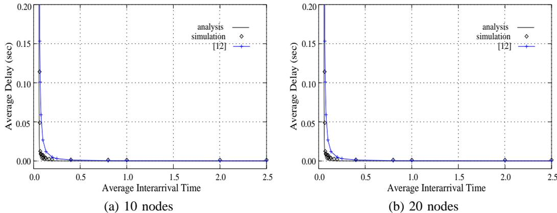
Fig. 3. Comparison of the average packet delays.
