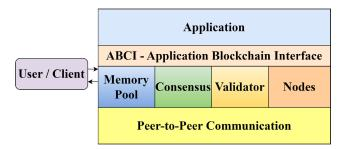
FIGURE 7. Structure of the tendermint core.
