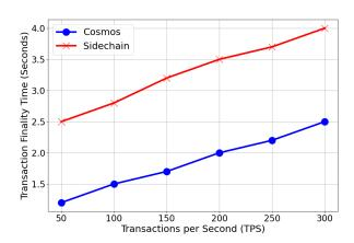
FIGURE 12. Comparison of transaction finality time between cosmos and sidechain networks as transactions Per Second (TPS) increase.
