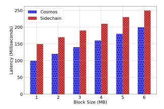
FIGURE 14. Comparison of latency between cosmos and sidechain networks for different block sizes (MB).
