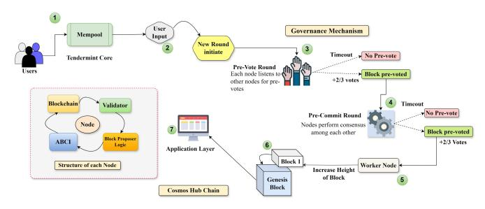
FIGURE 8. Visualizing the interaction between cosmos blockchain components, this flow illustrates nodes collaborating as a network of interconnected chains.
