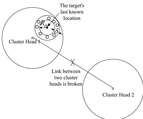
Fig. 2. 2nd level of failure recovery
