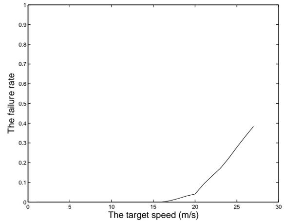
Fig. 4. The tracking failure rate of LTTP with 0.1s as the tracking resolution
