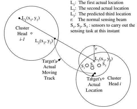
Fig. 1. Handover of target tracking among sensor triplets
