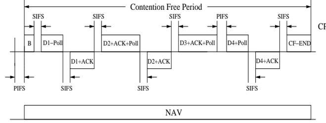
**Fig. 2.** PC to station frame transmissions in PCF.
