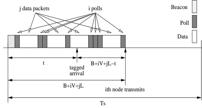
**Fig. 3.** Packet delays when arriving packet finds an empty queue.
