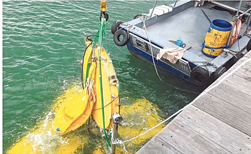
A 300kg underwater acoustics camera, built by researchers from the National University of Singapore's Tropical Marine Science Institute, being deployed near St John's Island last year. Sound is a good indicator of coral reef health. According to a British study, healthy reefs are three times louder than degraded ones.
