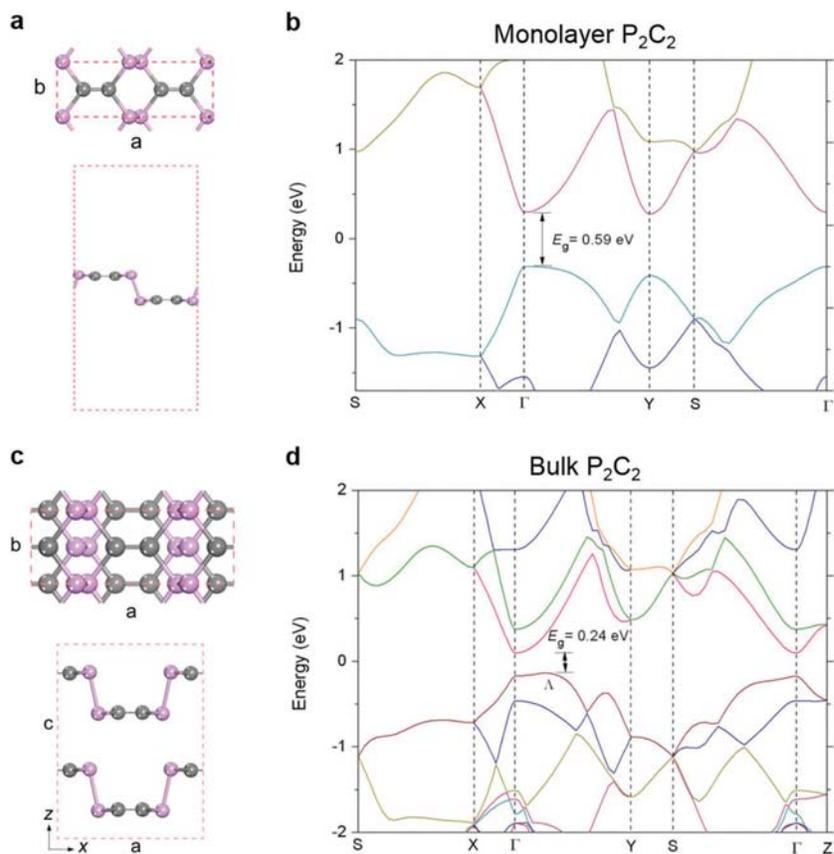
**Figure 1.** DFT Calculations of monolayer and bulk  $\text{P}_2\text{C}_2$ . a) The top and side views of the monolayer  $\text{P}_2\text{C}_2$  sheet. b) Band structure of the  $\text{P}_2\text{C}_2$  sheet. c) The side and top views of the bulk  $\text{P}_2\text{C}_2$ . d) Band structure of the bulk  $\text{P}_2\text{C}_2$ . Note that the peak of the valence band is at the  $\Lambda$  point between  $\Gamma$  and Y points.
