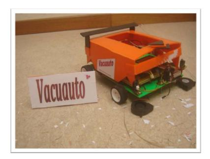
Knowing the energy diverted to a simple task or cleaning floors and sweeping, our group channelled our efforts in designing a device that could do all that and more. 'Vacuauto' we named it, being the combination of the effectiveness of vacuuming and the effortless ease of automation. With minimal wiring, two layered PCBs and best of all, only the usage of one PIC, our group has designed in a few weeks, one of the most robust projects of this semester.
