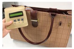
The central subsystem is the core of the system which links up the other subsystems and also provides reminders and helps track personal expenditure. The console is easily removed from the side pockets and fits comfortably in one's hands.
