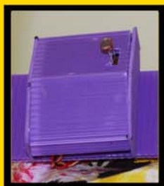
Light sensor sets cover orientation based on external light intensity
