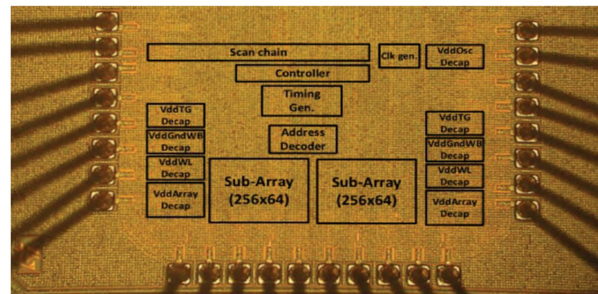
Fig. 3. RazorSRAM chip micrograph, as published at ISSCC
