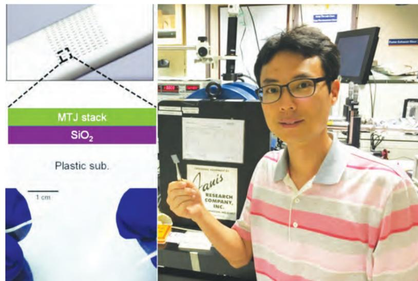
**Top left inset:** Optical images of the magnetic memory devices after the transfer onto a flexible plastic platform with a schematic diagram of an individual memory unit.
