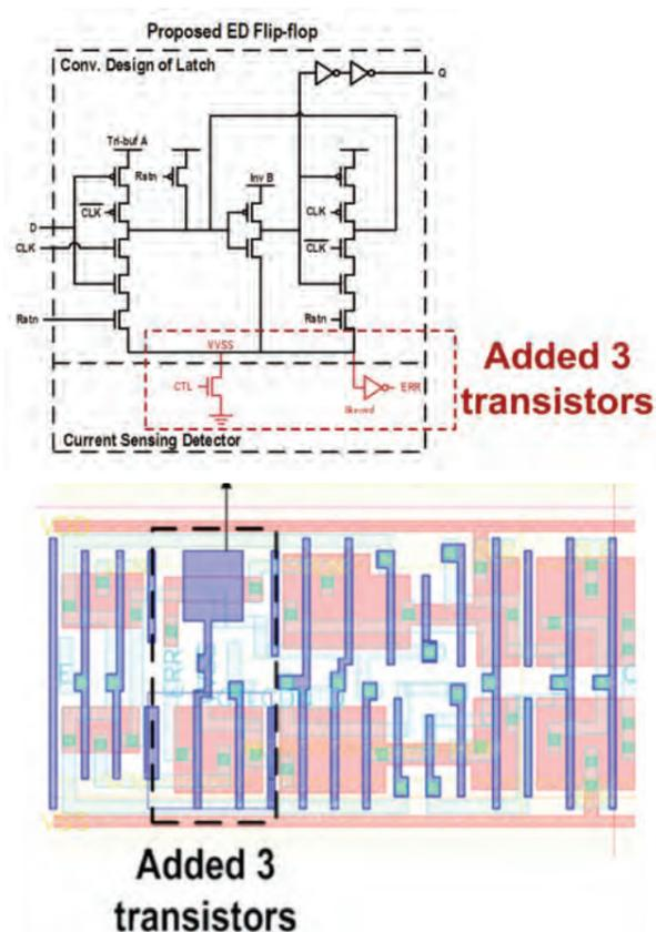
Fig. 1. The iRazor concept: Only three additional transistors per sequential element are needed (circuit on the top, physical layout at the bottom)
