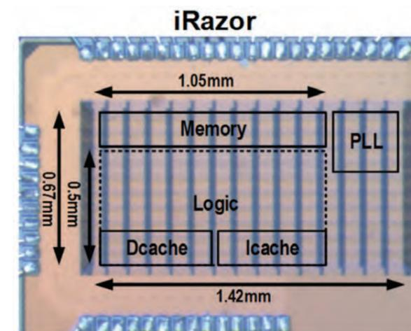
Fig. 2. iRazor chip micrograph (ARM Cortex-R4 microprocessor), as published at ISSCC
