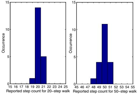
Fig. 6. Histograms of the digital step counter output.
