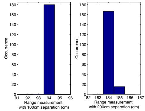
Fig. 8. Histograms for range measurement with 1m (left) and 2m (right) separations.
