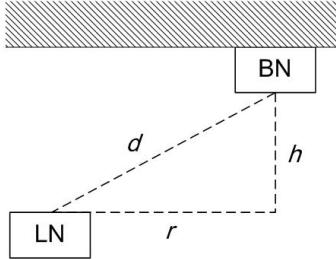
Fig. 4. Original and projected range measurements.
