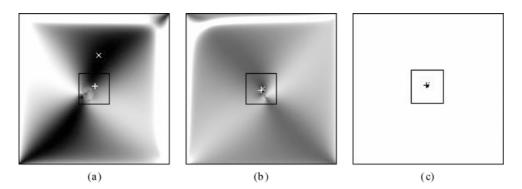
*Figure 15.* Residual error images resulting from using features in different regions in the COKE image. Figure (a) was obtained by using features from the bottom-left and (b) from the bottom-right quarter of the image plane respectively. Figure 15(c) was the binary image obtained by performing an intersection of the thresholded version of (a) and (b).
