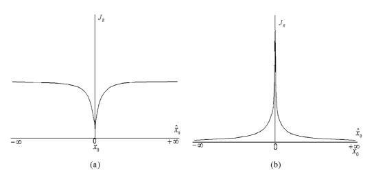
*Figure 4.* Error profiles of the bas-relief valley in the limiting cases. (a) The true FOE coincides with the origin and (b) The true FOE lies at infinity.
