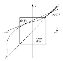
*Figure 5.* Geometry of the bas-relief valley when the distribution of feature points is uneven, with centroid at  $(\tilde{x}, \tilde{y})$ . The solid line corresponds to the bas-relief valley; the dashed line corresponds to the bas-relief valley if the feature points are evenly distributed; the dotted line is the line passing through  $(\tilde{x}, \tilde{y})$  and  $(x_0, y_0)$ .
