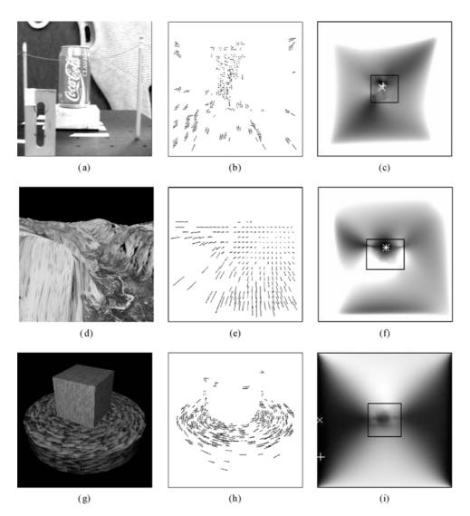
*Figure 14.* Residual error images for real image sequences. Each row corresponds to one image sequence. From top to bottom: COKE, YosemiteNoCloud and SOFA1. For each row, an actual image of the sequence, the optical flow field and the residual error image are shown from left to right. True FOEs and global minima of the residual error surfaces were highlighted by "+" and " $\times$ " on the residual error images respectively.
