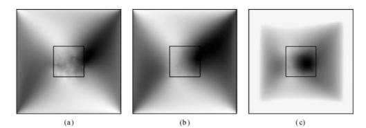
*Figure 11.* Residual error images for the flow fields with anisotropic noise. Numbers of feature points were 200 for (a), 2000 for (b) and  $\mathbf{v} = (1, 1, 1)$  for (a) and (b). For (c), number of feature points was 800, and  $\mathbf{v} = (0, 0, 2)$ .  $\mathbf{w} = (0, 0.0005, 0.001)$  and noise level was 50% for all the images.
