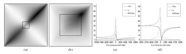
*Figure 7.* Influence of the FOV on the residual error images.  $\mathbf{v} = (1, 1, 1)$  for both (a) and (b); FOV was 28° for (a) and 90° for (b). Figures (c) and (d) correspond to the residual profiles of the bas-relief valleys in (a) and (b) respectively. Notations as before.
