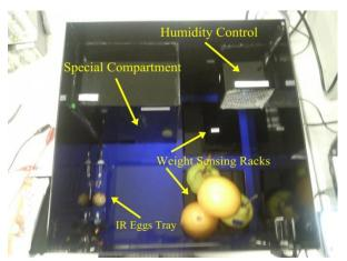
The Smart Fridge has 3 ways of taking stock of items. First is using Force Sensitive Resistors to gauge the weight of items placed on designated Racks. Secondly, RFID tags are attached to an item; it is then tapped against a RFID Reader before adding into the fridge. Thirdly, the user can add the item into the fridge and then update the inventory through the user interface.
